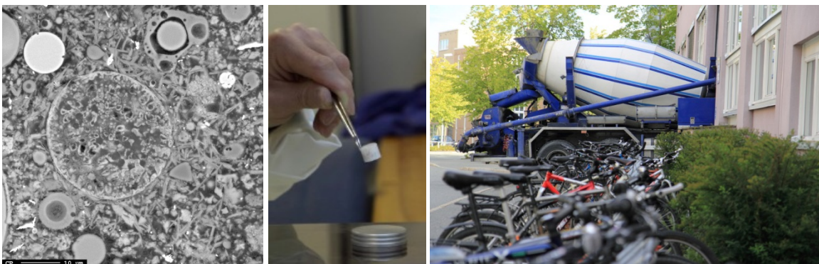
Testing from small to full scale: To the left: Scanning Electron Microscope (SEM) image of cement paste with fly ash, In the middle: Thermogravimetric analysis (TGA) and to the right: Delivery from concrete-mixer truck in the laboratory at SINTEF/ NTNU. Photos by Giedrius Zirgulis
