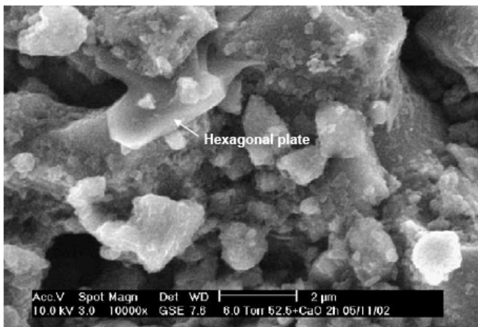
Fig. 10 ESEM (Environmental Scanning Electron Microscope) micrograph of paste with 3 % CaO after 2 h of curing.
