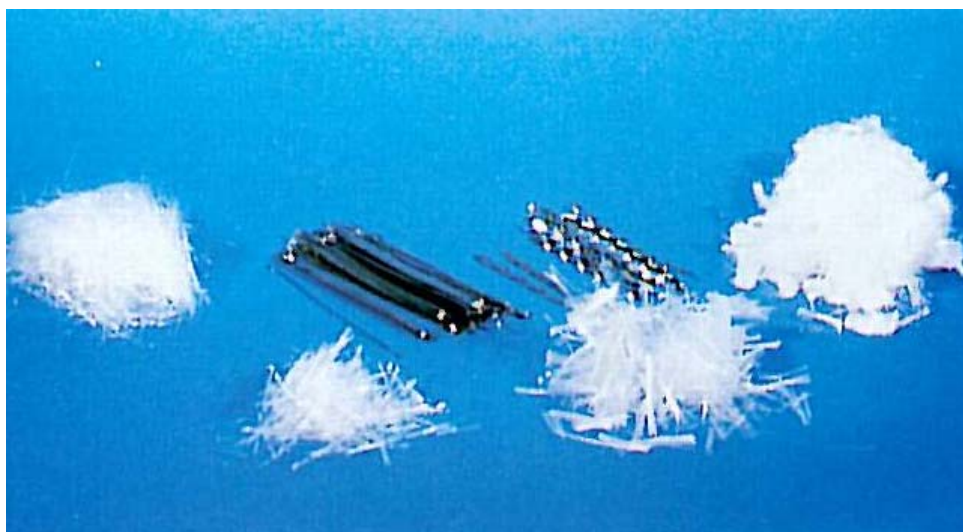
Figure 1: Steel, glass, synthetic and natural fibres (ACI 544.1R-96 1997)
