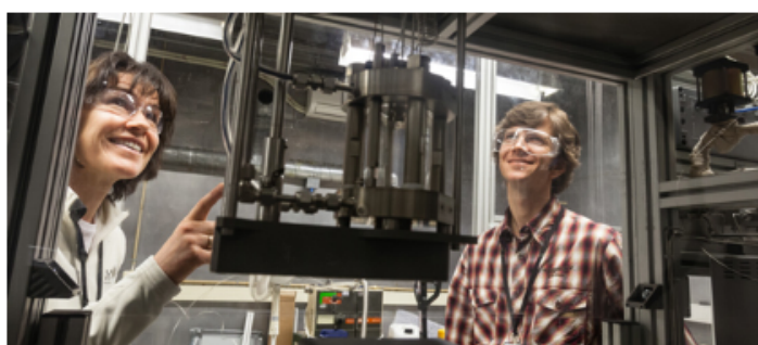
Mona J. Melnvik (IMPACTS Coordinator) and Svend Tollak Munkejord demonstrating the CO 2 mixture phase equilibrium cell at SINTEF Energy Research. (Photo: Thor Nielsen/SINTEF)
