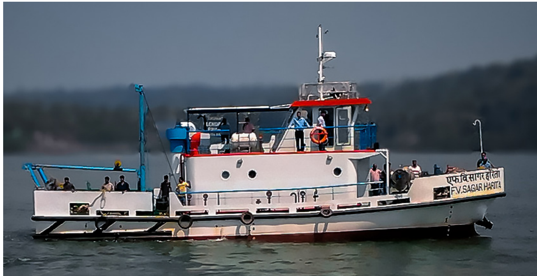
F.V.Sagar Harita- Long Liner Cum Gillnetter - Designed by CIFT and constructed by Goa Shipyard Ltd- RSW tanks : 1.2 cu m each: 2 no.s
