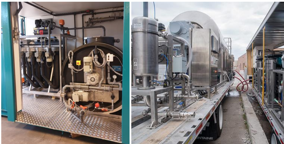
Figure 5: Left: Ice slurry system in a transportable container (Vikse, 2023). Right: Mobile unit that can deliver to different plants and harvesting sites (Deepchill, 2023).
