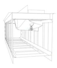
The large windows will allow alternative measurement techniques such Particle Image Velocimetry (PIV), Laser Doppler Velocimetry (LDV) and Digital Image Correlation (DIC), thus expanding the range of services that the cavitation tunnel has traditionally offered such as cavitation observations, pressure pulses and noise measurements.
