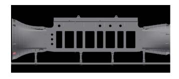
The new model configuration with the motors installed inside models will enable running several propulsors at the same time and hence allowing complicated propulsive setups to be tested.
