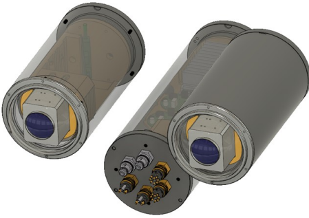
Figure 43: Render of the stereo camera
