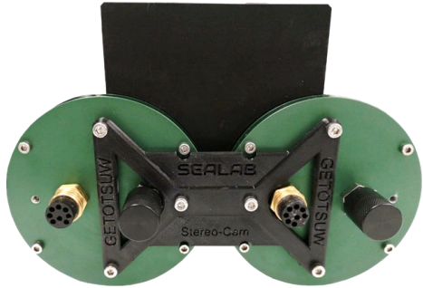
Figure 49: Connector interface for the stereo camera
