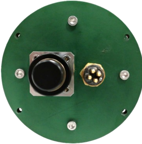
Figure 47: Main pod connector interface towards the topside umbilical
