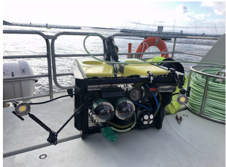
Figure 53: Stereo camera integrated on the ROV
