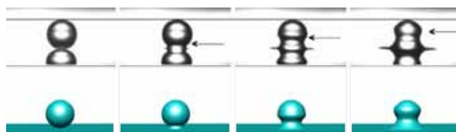
Comparison of experiments and modelling falling drops on a water surface, and the coalescence process itself between a drop and the water surface. Figure from Knut Erik Teigen, NTNU. The upper part is published with permission from Xiaopeng Chen, Physics of Fluids , 18, 051705 (2006). Copyright 2006, American Institute of Physics
