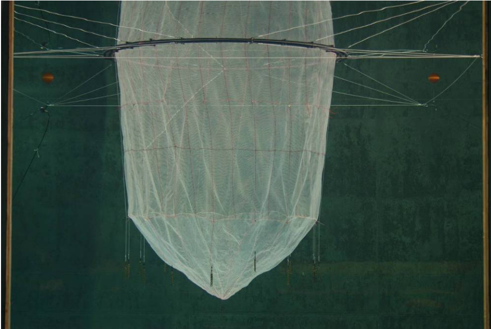
Figure 6 Model scale test of net cage by Egersund Net.
