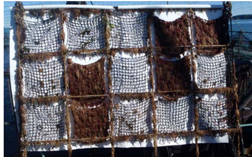
Figure 4 Example of the fouling distribution on coated nets with different Cu 2 O concentrations.
