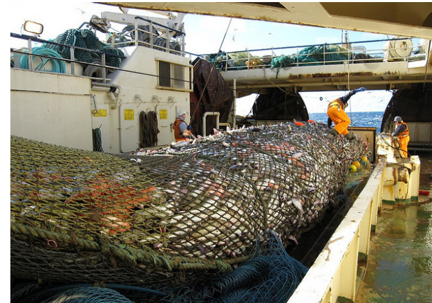
Grid-covered method + blinded codend
