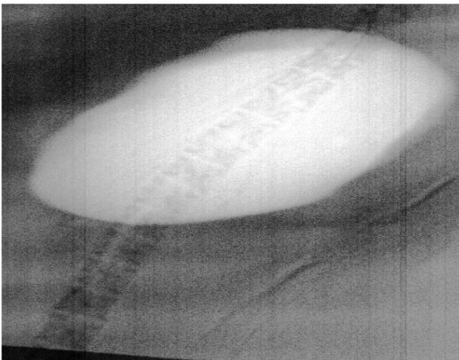
Figure 26: 5 kg fish imaged at 160 kV and 6 mA; The integration time is 10 ms
