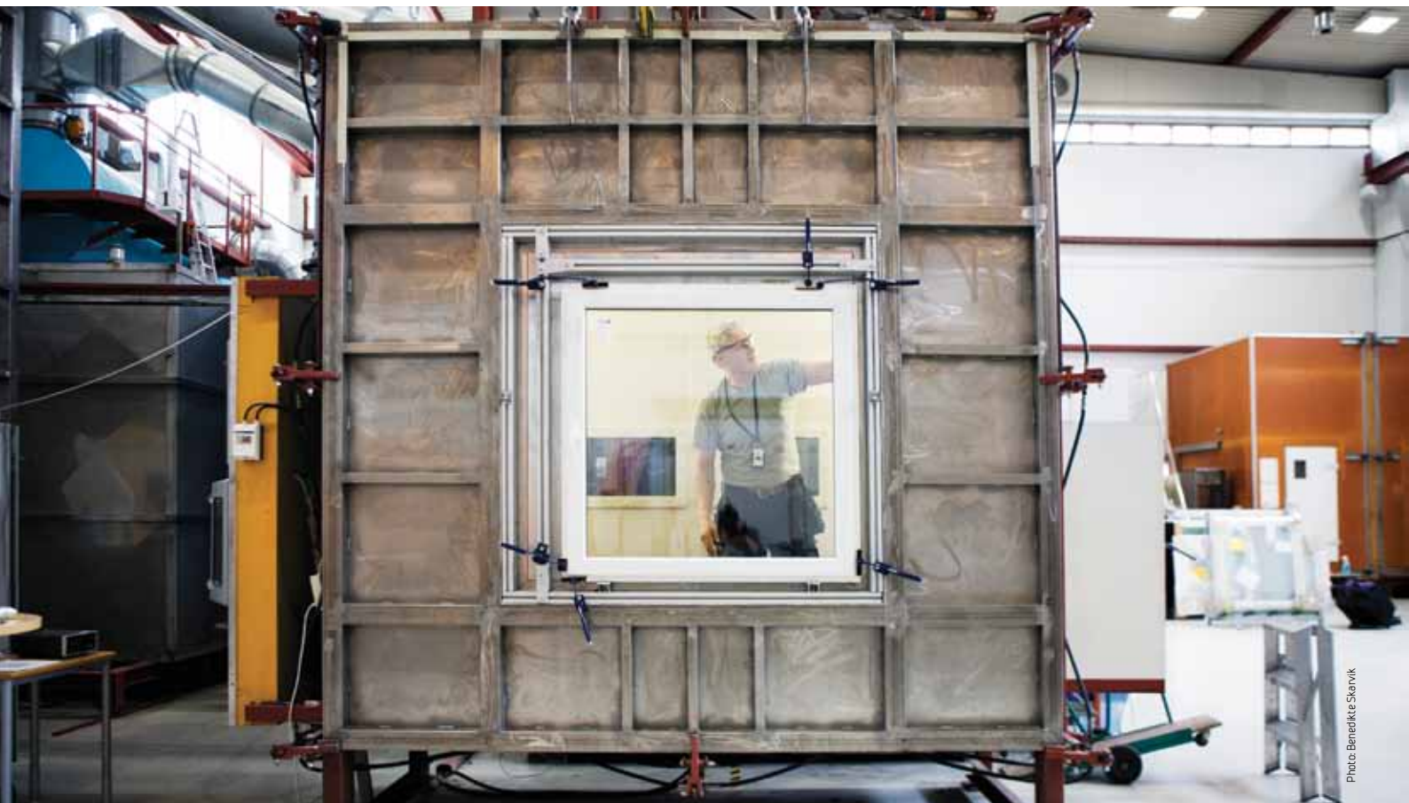
Senior technician Øystein Holmberget tests window air- and rain-tightness.
