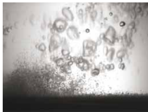
Multiphase flow experiments. Sand settling in middle of slug body.
