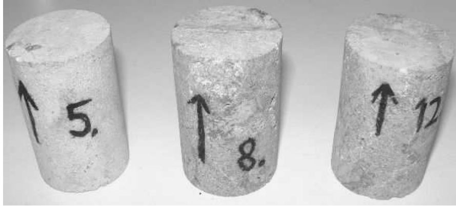
Fig. 5. Three core plugs with diameter of one and a half inches, and a height of five centimetres.
